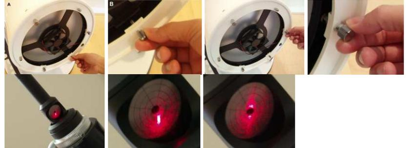
**STEP 8: Iteration adjustments on both mirrors**
