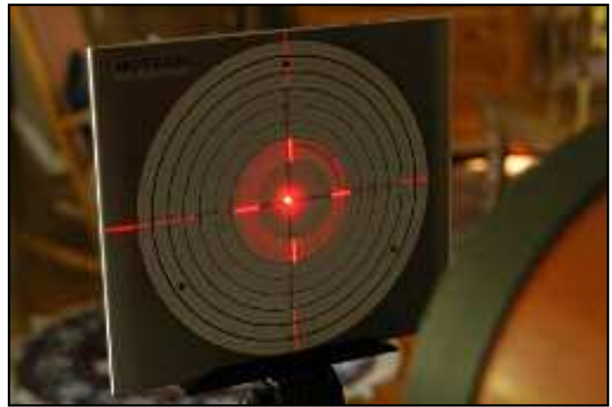
Left: To verify the visual back or focuser is parallel with the optical path, rack the focus in and out. The three laser spots should expand from a single point, but remain centered on the target crosshairs. Right: This is what you will see if the collimator is properly aligned with the telescope but the secondary mirror is offset. The central doughnut is not centered in the middle target ring of the collimator face. To center the secondary, the corrector plate is shifted within its mounting cell.
