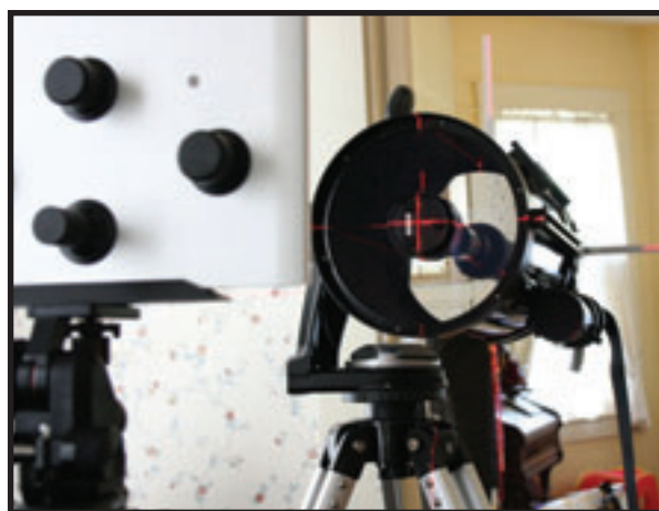
Image 8 - Aligning the Advanced CT Laser Collimator with help of the alignment tabs.
